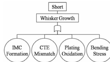
Fig. 3. Fault tree of electrical short circuits due to whisker growth with stresses.
