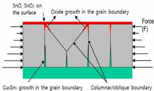
Fig. 4. Sn moving along the grain boundary of plating.
