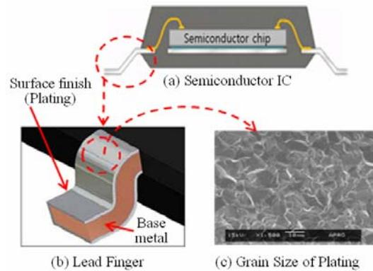
Fig. 1. Lead finger and its plating grain structure for semiconductor IC.
