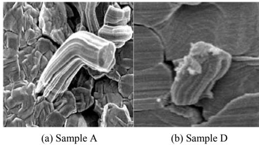
Fig. 10. Whisker growth along plating grains at 2,000 cycles.
