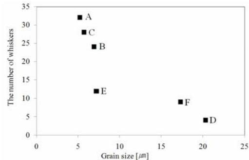
Fig. 9. Relation of plating grain size to the number of whiskers.
