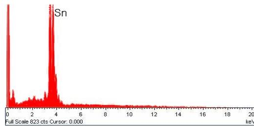
Fig. 8. Elements analysis of whisker using EDX.
